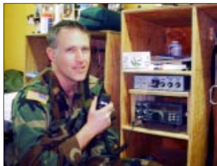
T9/KC5YOR operated his TenTec Delta II transceiver out of his quarters, feeding his roof-mounted dipole with 450-Ω ladder line.
